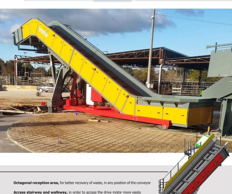
Raised edges, on the maintenance way side, to avoid any overflow on the maintenance way (Yellow color on the sketch)
