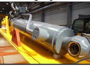
3 identical and interchangeable hydraulic cylinders
